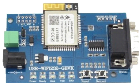
Figure 24 USR-WIFI232-S/T/G2/H Evaluation Kit
